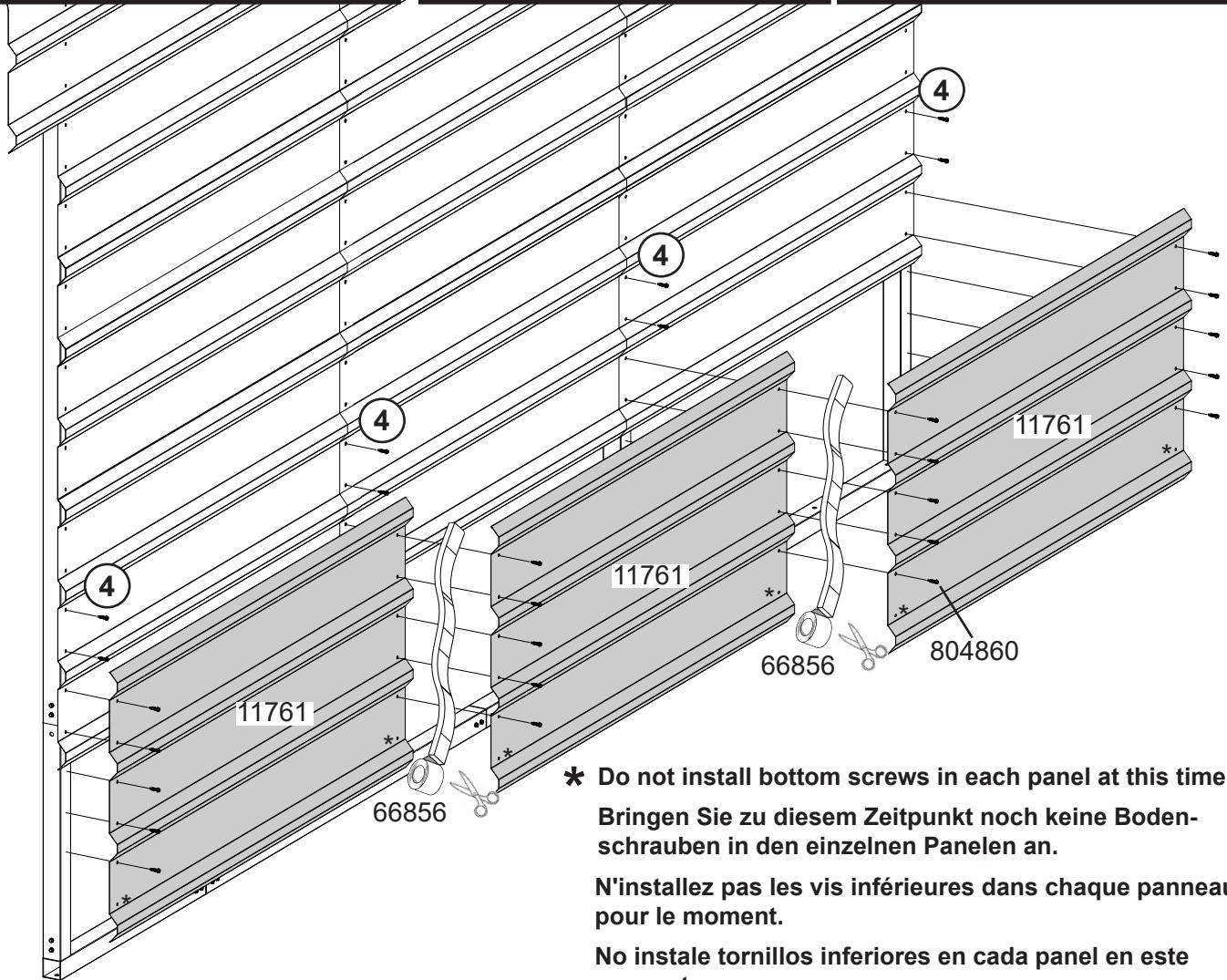
\* Do not install bottom screws in each panel at this time.
