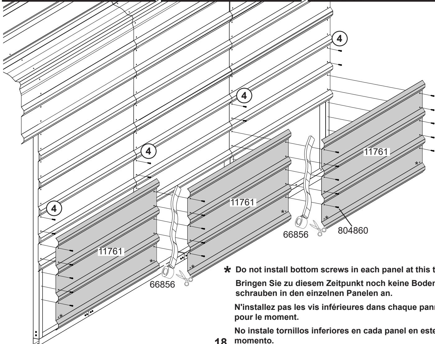
**\* Do not install bottom screws in each panel at this time.**
