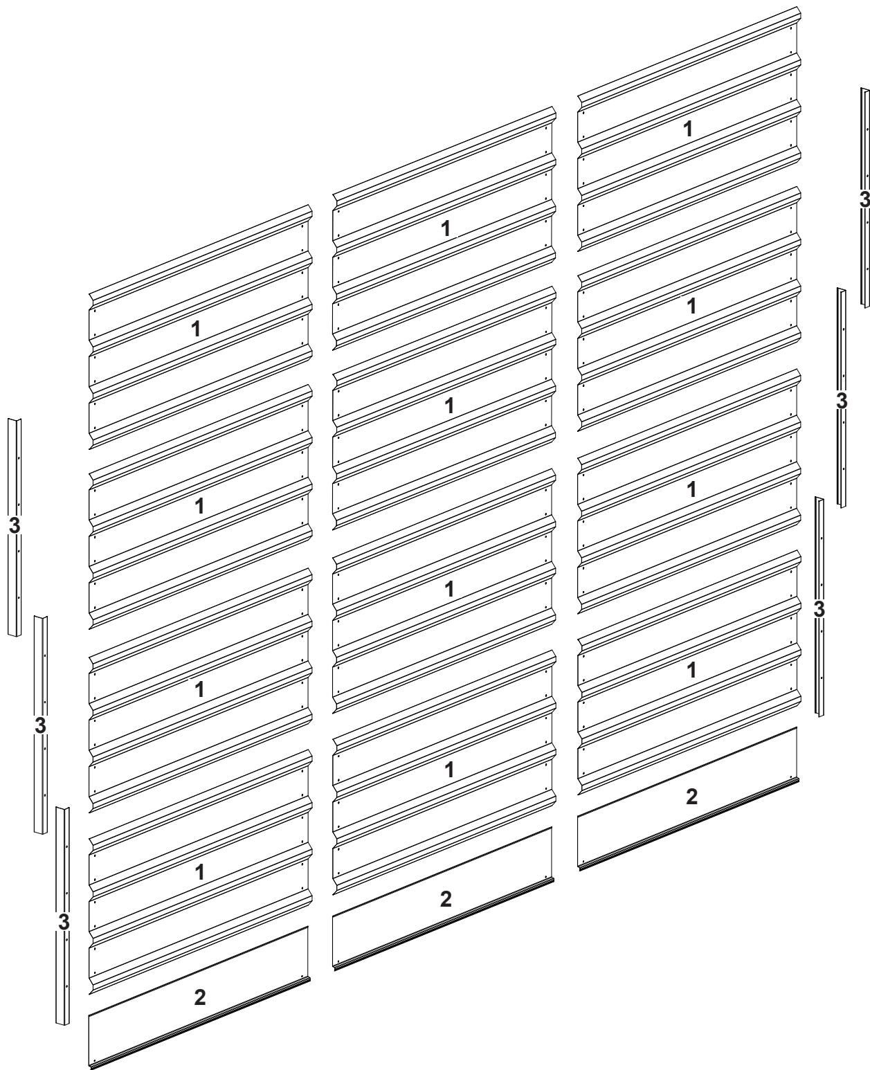
**NOTE:** Buildings longer than 15' will receive 1 additional box for each 4.5', four middle panels and one bottom panel. These panels are inserted in the middle section of the base building.
